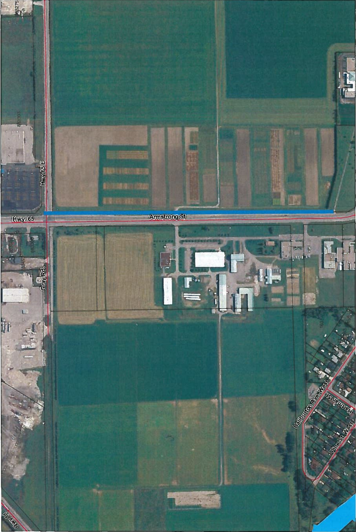
Armstrong Street – ARIO property to Highway 65E - (2.5 metres width constructed / paved lane) 660 m
