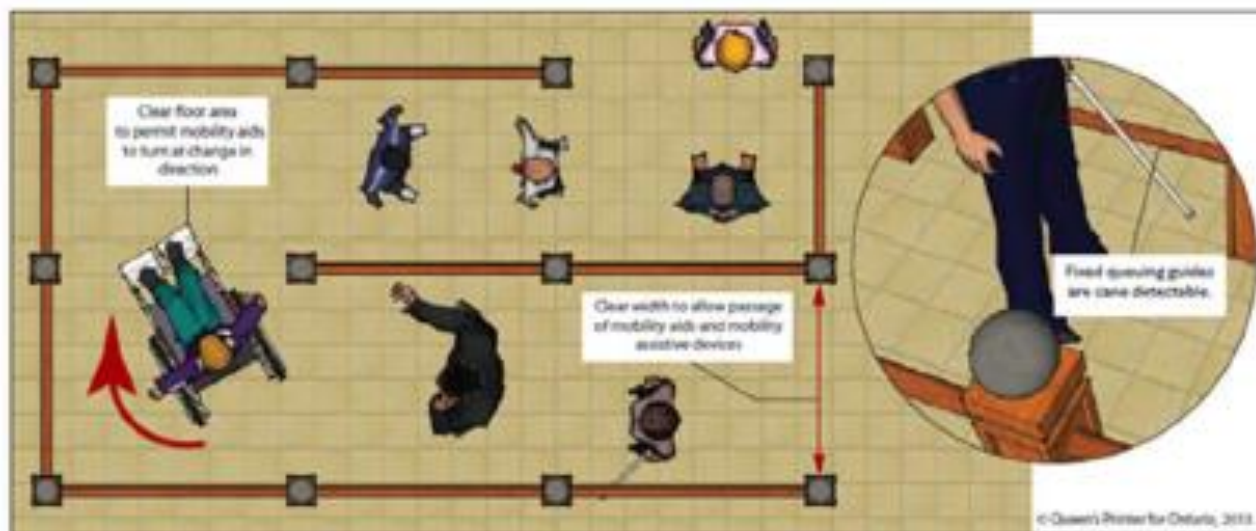
Figure 16 - Accessible fixed queuing guides
