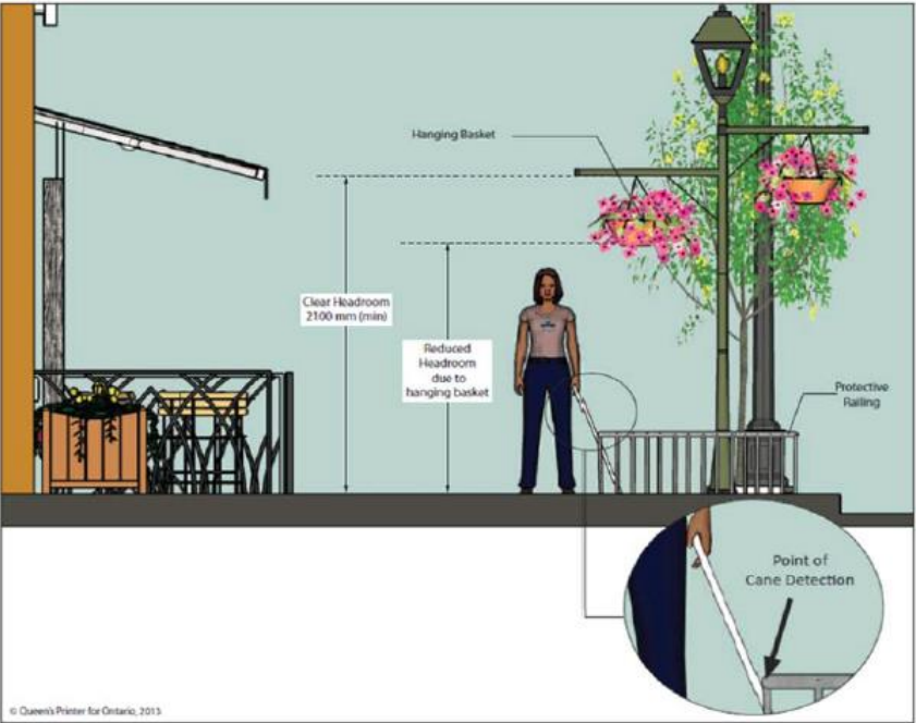
Figure 8 - Minimum head room clearance
