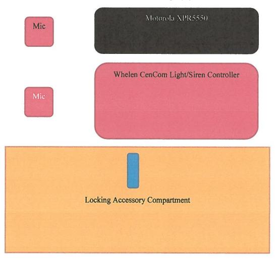
The top of the console shall be easily removable for maintenance and service. The console shall have storage bin with a grey painted finish installed between the driver and passenger seats for storage of 12 volt or 110 volt chargers etc., and shall c/w lift up stainless steel access door. Two (2) 110 volt duplex receptacles shall also be mounted.
