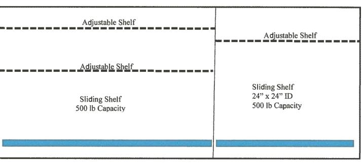
Maximum Height 36" – 38" from command floor The top of this compartment will be used in the command canopy as a teble top.
