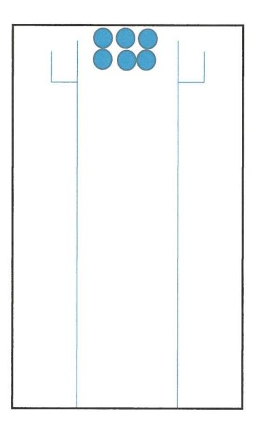
**REAR OF RESCUE BODY, FACING CASCADE** Vehicle shall be equipped with a 24" wide x 12" deep shelf with a 1" lip mounted around shelf, shall be located directly above the cascade bottles.
