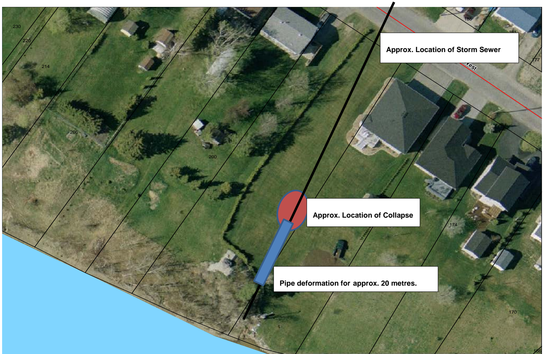
Approximate Location of Storm Sewer Failure – 182 Pine Street West.
